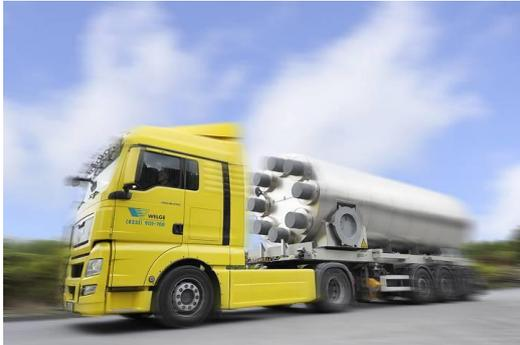
Heat storage tank transported by truck
