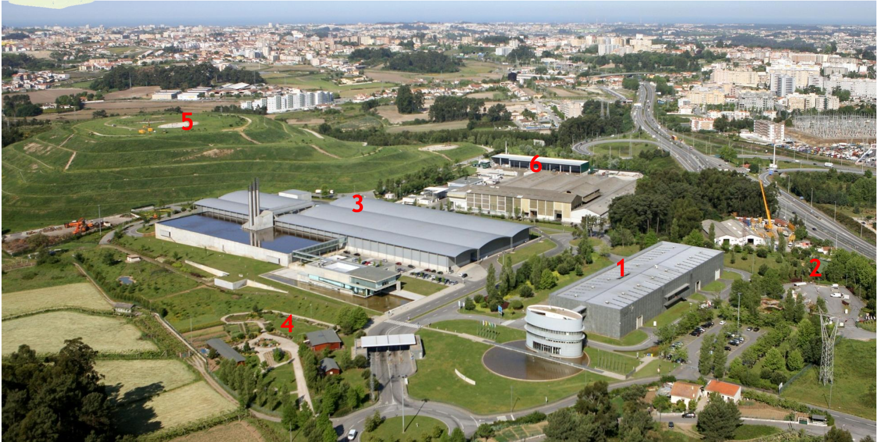
LIPOR, Baguim do Monte (Portugal) – Sorting Plant(1), Drop off Site (2), Composting Plant(3), Horta da Formiga – Home Composting Centre (4), Adventure Park(Ermesinde Old Landfill) (5), Platform (6)
